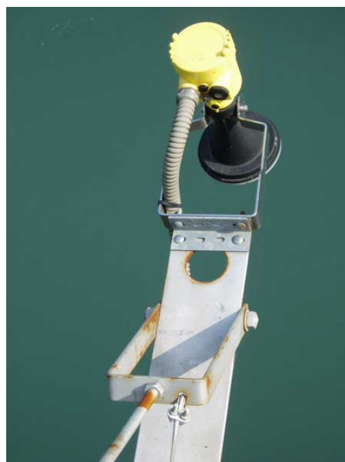
Figure 5. Level measurement by emerged radar. [© EDF DTG]
