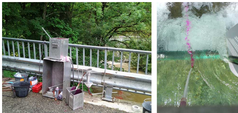
Figure 9. Left: Rhodamine injection device. Right: Rhodamine enters the stream. The tracer (harmless to fauna and flora) does not colour the water. Its dilution is then analysed by a fluorimeter (measuring the attenuation of its fluorescence), still today in the laboratory; tomorrow can be directly in the field [© EDF DTG]
