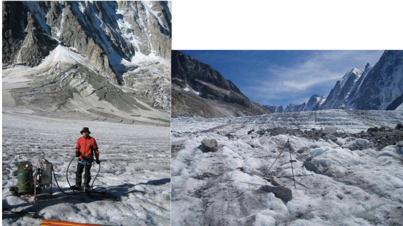
Figure 4. Late winter coring in the Alps (Mont Blanc massif) using a manual corer (left). The cores are then weighed to transform the snow depth into water depth (right). [© Ch. Vincent]
