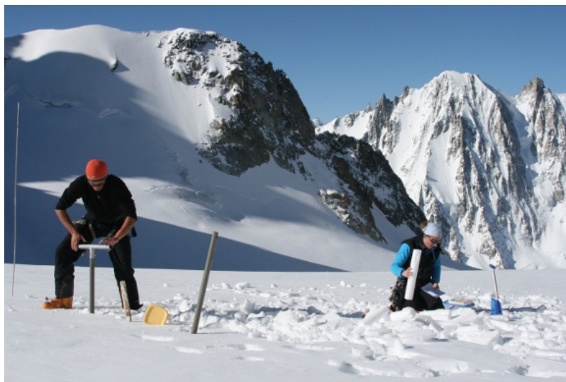
Figure 3. Late winter coring in the Alps (Mont Blanc massif) using a manual corer (left). The cores are then weighed to transform the snow depth into water depth (right). [© P. Ginot]
