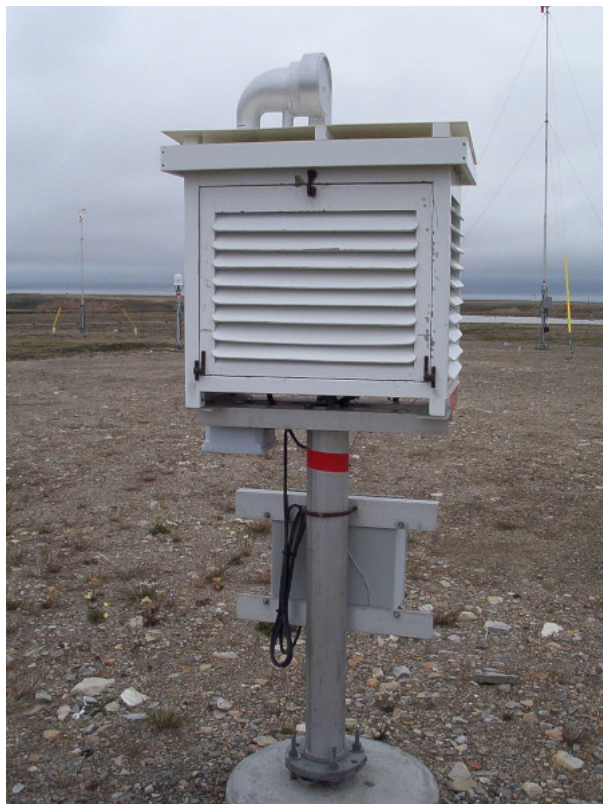
Figure 2. Stevenson shelter containing in particular a thermometer for measuring air temperature. The shelter is designed to protect the thermometer from solar radiation, thermal radiation from the ground and the sky, and possible precipitation. (See "Ground Weather Observations: What are we measuring and what do we do with them?") [Source: Public Domain]
