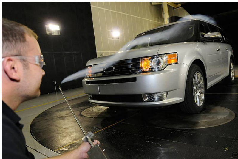
Figure 11. In a wind tunnel, use of an opaque gas to visualize the influence of the shape of the automobile on the flow and to test the possibilities of reducing the CX drag coefficient. [Source: By Ford Motor Company from USA (Flex Aerodynamics)[CC BY 2.0 ( http://creativecommons.org/licenses/by/2.0 ) or CC BY 2.0 ( http://creativecommons.org/licenses/by/2.0 )], via Wikimedia Commons]
