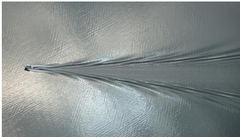
Figure 8. Wake of a boat near the Froude limit, for which the wavelength of the waves is comparable to the length of the boat. [Source: By Edmont (Own work)]CC BY-SA 3.0 ( http://creativecommons.org/licenses/by-sa/3.0 ) or GFDL ( http://www.gnu.org/copyleft/fdl.html ), via Wikimedia Commons]
