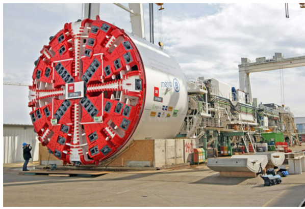
Figure 8. Example of a tunnel boring machine. Tunnelling machines are of several types depending on the ground they cross, at earth pressure, sludge pressure, air pressure. The pressure is intended to stabilize the slaughter front. They are real rail-based factories, extremely powerful. The main parts are essentially, in order: the cutting wheel, the conveyor belt for the rear excavated material, a shield if the ground is soft, push reaction cylinders on the wheel, the cone shaped exhaust skirt, the lining segment erector (prefabricated), storage wagons. Outside a sludge treatment plant if sludge pressure. [© PHOTOPQR/LE PROGRES/PHILIPPON JOEL]
