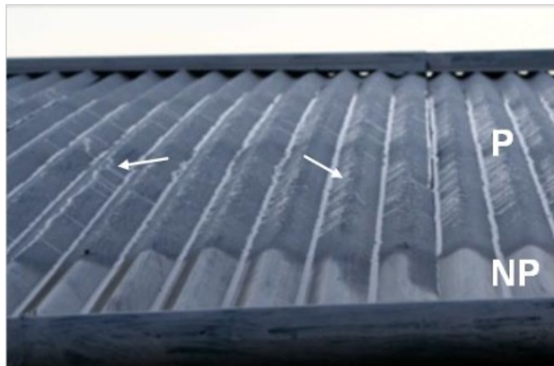
Figure 4. Drops sliding on the corrugation galvanized iron roof in Combarbala (Chile) with small tilt angle ( >15^\circ ). P: Painted part with additives (OPUR [12]) where dew forms and drop slide down on the corrugations (arrows). NP: Non painted part where dew does not form. [Source : J.-G. Minonzio].
