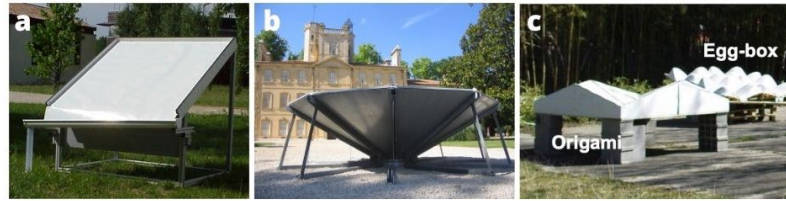
Figure 3. Various dew collectors: a : Plane; b : Cone [Source : Photo O.Clus] ; c: Origami and “egg-box” [Source : Photo D.Beysens].
