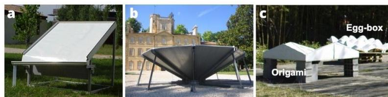
Figure 3. Various dew collectors: a: Plan; b: Cone [Source: Photo O.Clus]; c: Origami and egg-box [Source: Photo D.Beysens]
