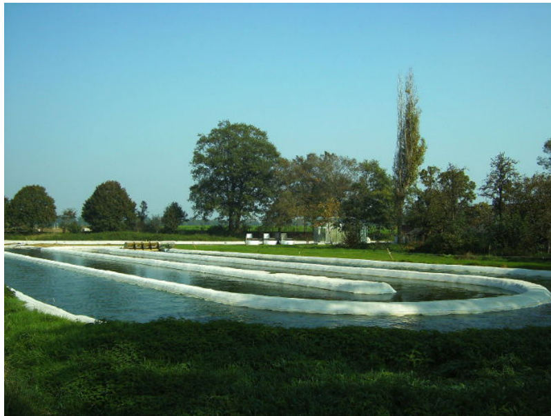
Figure 8. Open pool used for the culture of microalgae. The water is constantly kept in motion by a motorized paddle wheel. [Source: Photo by JanB46 [CC BY-SA 3.0], from Wikimedia Commons]
