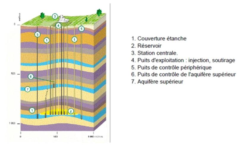
Figure 2. Cross-section of aquifer storage. [© Storengy]
