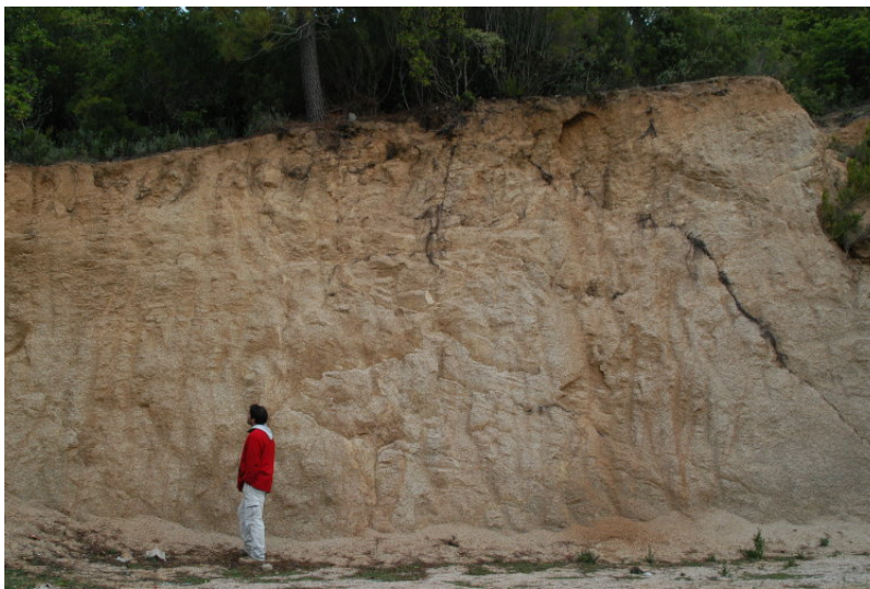
Figure 6. Outcrop of the saprolite of a granite in a quarry. Sartène region, cortica. [Source: © W. Wyns]
