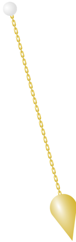
Figure 4. Simple pendulum. Almost all the mass is concentrated at the lower end in the conical shape that oscillates by sweeping an arc of a circle centred on the attachment point at the top of the chain. [Source: pixabay]
