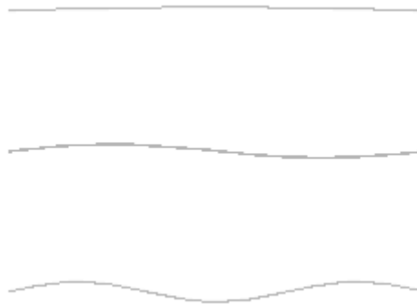
Figure 6. Oscillation of a vibrating string between two fixed points: fundamental mode and two first harmonics [Source: By Christophe Dang Ngoc Chan (cdang) (Own work)[GFDL ( http://www.gnu.org/copyleft/fdl.html ) or CC-BY-SA-3.0 ( http://creativecommons.org/licenses/by-sa/3.0/ )], via Wikimedia Commons]
