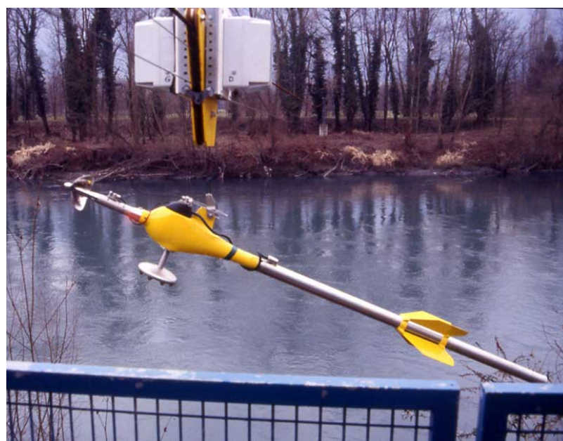
Figure 6. Hydrometric reel implemented at Grenoble Campus sur l'Isère station. [© LTHE, now IGE]
