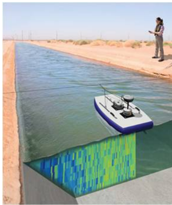
Figure 8. The ADCP velocity measurement is based on the pulsed Doppler principle: emission of ultrasonic pulses into the water and analysis of the frequency offset of the backscattered echo of the suspended particles. The device generally has 3 or 4 transducers emitting divergent acoustic beams around the vertical, which allows the vertical profile of velocities to be measured in three dimensions. [© EDF DTG]
