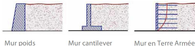
Figure 6. Evolution of retaining walls.
