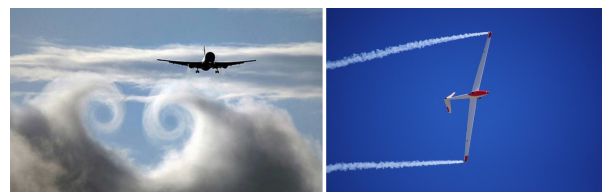
Figure 7. Illustration of marginal eddies at wingtips. On the left, the winding of these eddies generated by a large aircraft is made visible by the cloud below it. On the right, at the ends of the wings of a glider, these eddies are made visible by a condensation phenomenon located near their axis [Source: (left image) DR. (right image) Pixabay]
