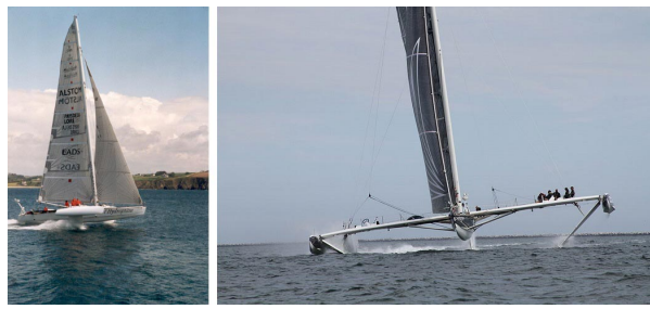
Figure 10. Hydrofoil sailboat built by Alain Thébault for sailor Eric Tabarly from an 18.24 m long Tornado trimaran hull. The thin legs that connect the side shells to the wing are made of titanium, the height of the mast, also made of titanium, is 27 m. This hydrofoil broke the speed record over a distance of 500 m in September 2009: 51.36 knots, or 95.3 km/h, with a top speed of 55.5 knots, or 103 km/h. [Source: (left photo) By Ludovic Peron (Personal photo)[CC BY-SA 2.5 ( http://creativecommons.org/licenses/by-sa/2.5 )], via Wikimedia Commons. (right photo) By Thomas Lesage (Own work)[CC BY-SA 3.0 ( http://creativecommons.org/licenses/by-sa/3.0 )], via Wikimedia Commons]
