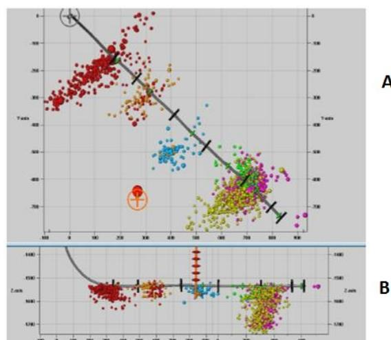
*Figure 4. The location of the induced micro-seismic activity allows the extension of hydraulic fractures to be mapped. (A) Top view; fractures are perpendicular to the borehole. (B) Cross-section view in a vertical plane showing the geometry of the horizontal borehole and the location of the micro-seismic sensors (vertical orange structure). [Source: Diagram, S. Maxwell, Schlumberger]*
