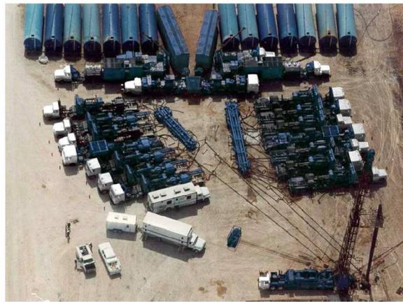
*Figure 3. A hydraulic fracturing operation as carried out for non-conventional hydrocarbon exploitation. At the bottom we see the water tanks ready for an injection of about 500 m<sup>3</sup>. The drill head is visible in the lower right corner of the image. The trucks in front of the tanks prepare the fluid-sand mixture which is injected by the two rows of truck-mounted pumps. Each pump has a power of about 500 hp. [Source: Photo Schlumberger]*
