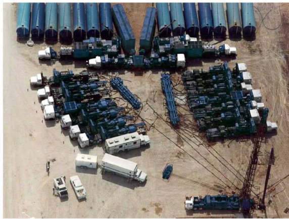
Figure 3. A hydraulic fracturing operation as carried out for non-conventional hydrocarbon exploitation. At the bottom we see the water tanks ready for an injection of about 500 m 3 . The drill head is visible in the lower right corner of the image. The trucks in front of the tanks prepare the fluid-sand mixture which is injected by the two rows of truck-mounted pumps. Each pump has a power of about 500 hp. [Source: Photo Schlumberger]
