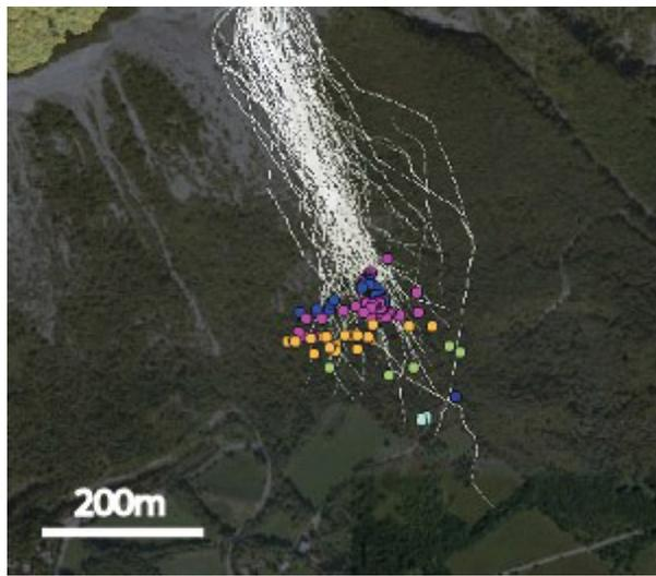
*Figure 7. Example of a rockfall simulation: the white traces represent the simulated paths of the blocks; the colored points represent the collapsed blocks observed on the slope. (software used: Rockyfor3D)*
