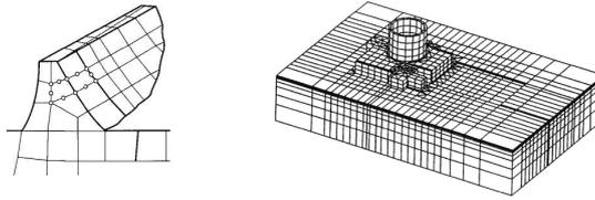
*Figure 5. Meshing of 2 structures in finite elements. On the left, a dam (very simplified) and its valley. On the right is a power station and its nearby site. The method consists in writing the mutual equilibrium and deformations of a large number of small volume elements, each made of materials with their own rigidity and strength. [Source: MESTAT, P., (1997), Finite element meshes, advice and recommendations, BLPC 212, 39-64]*
