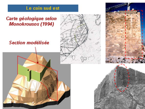
Figure 4. Numerical modelling (by the "Discrete Element Method") of the stability of the southeast corner of the Acropolis of Athens. [Source: PhD thesis of C. Lambert, coll. F. Darve, Grenoble INP]
