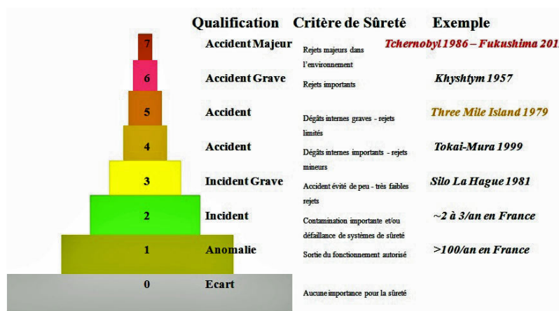
Figure 7. INES scale of nuclear accidents[Source: Bertrand Barré]
