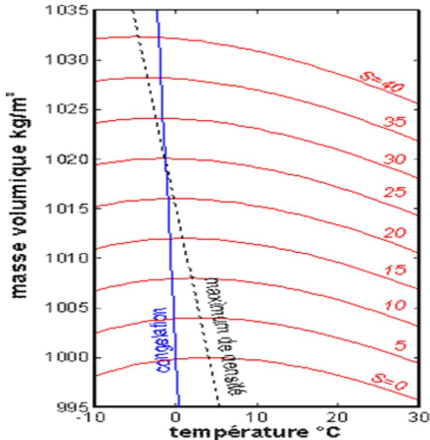
Figure 2. Variation of the sea water density with temperature for various values of the salinity.
