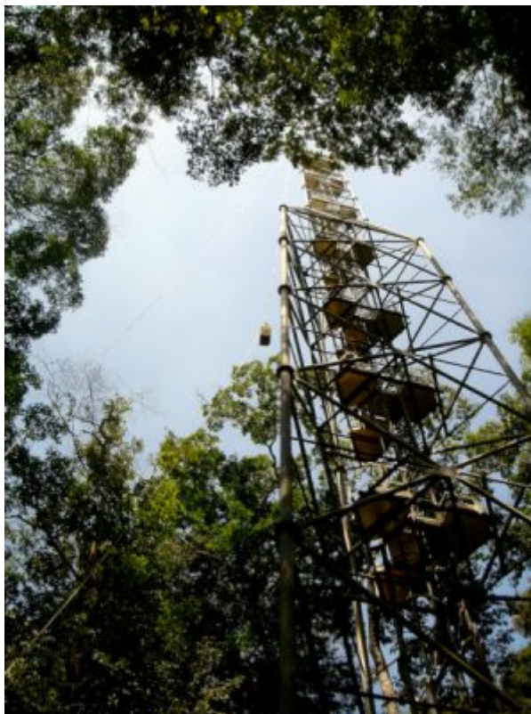
Figure 2. Flow tower to measure the gas exchange between the forest and the atmosphere (Paracou site in French Guiana). In the same area, ground-based sensors have been installed to assess GHG emissions, including NOx. [Source: © Alain Pavé]
