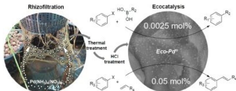
Figure 4. Microstructure of an Eco- Pd and its applications in organic synthesis. [Source: © C. Grison]
