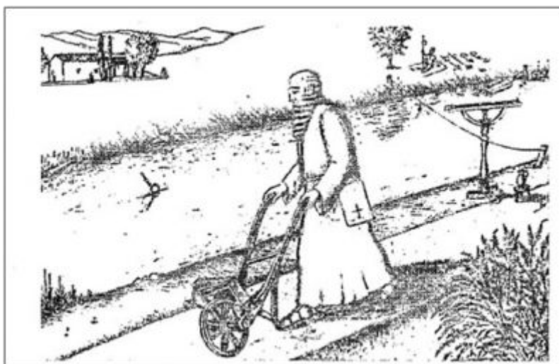
Figure 1. Surface velocity measurement by Leonardo da Vinci. [Source: reconstruction by Arthur H. Frazier]
