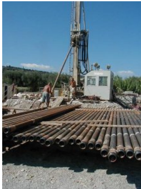
Figure 3. Example of a small drilling rig to reach a depth of 800 m. The drill pipes are placed here in front of the device. For greater depths, the rods are held vertically next to the drilling rig and are handled automatically. [Source: © F.H. Cornet]
