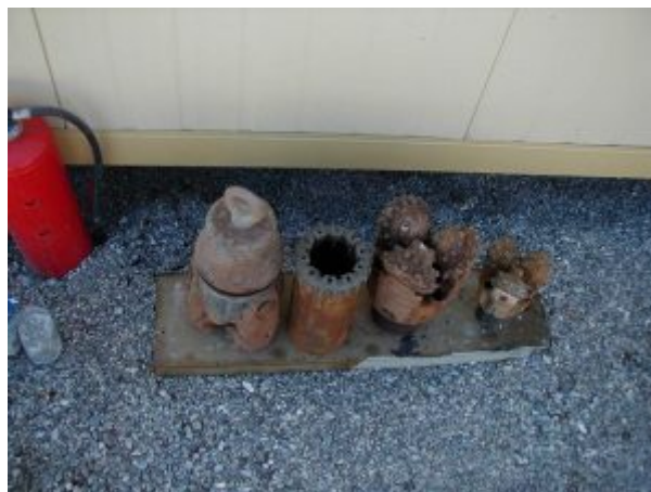
Figure 2. Examples of drilling tools. On the left is the corer used to produce the cores in Figure 6. On the right are two examples of wheel drills. [Source: © F.H. Cornet]
