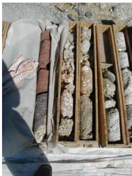
Figure 1. Example of rock cores. They are more or less cylindrical, depending on the alterability of the rock, but also according to the coring technique. For example, for very deformable materials, a double core barrel is used, of which only the outer part rotates with the drill string, while the central part remains free of any rotation. [Source: © F.H. Cornet]
