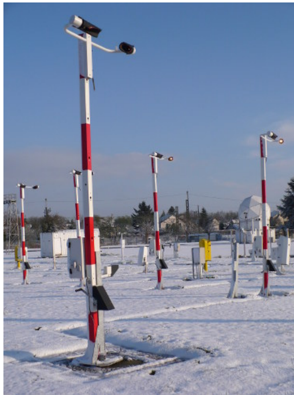
Figure 11. Diffusometers. [Source : © Michel Leroy]
