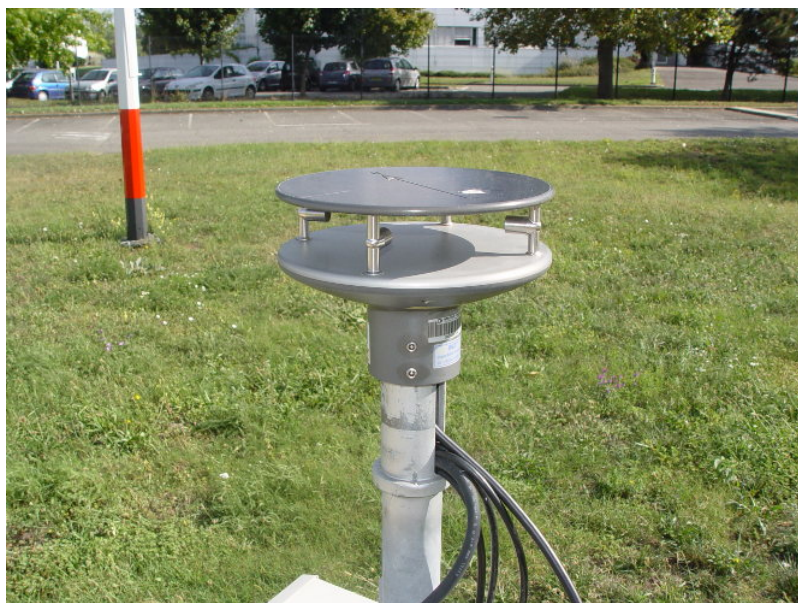
Figure 7. Example of an ultrasonic wind sensor. [Source : © Lantuejoul Pierre - Météo-France]
