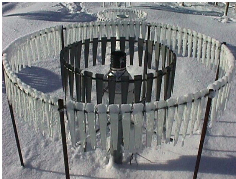
Figure 9. Rain gauge protected by a dual Alter display [National Center for Atmospheric Research, http://www.rap.ucar.edu/projects/marshall/Events/19MAR98/MVC-021F.html ]
