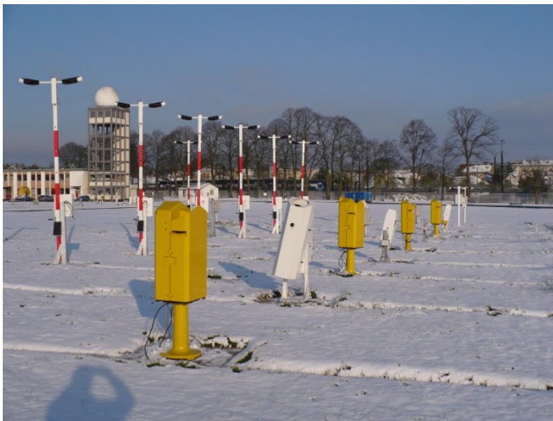
Figure 12. Cloud rangefinders. [Source : © Michel Leroy]
