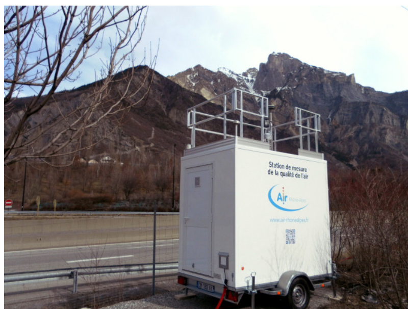
Figure 3. Mobile emission measurement station. [Source : Air Rhône-Alpes [CC BY-SA 4.0 ( https://creativecommons.org/licenses/by-sa/4.0/ )]]
