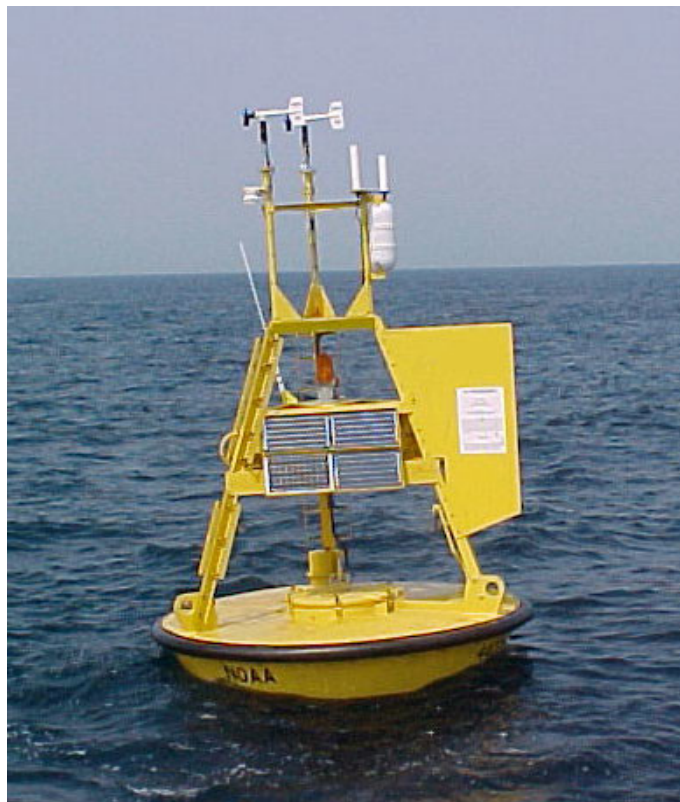
Figure 3. A 3-metre diameter moored weather buoy used by the U.S. Weather Agency. In particular, it is equipped with a thermometer for measuring sea surface temperature. [Source: Public domain]
