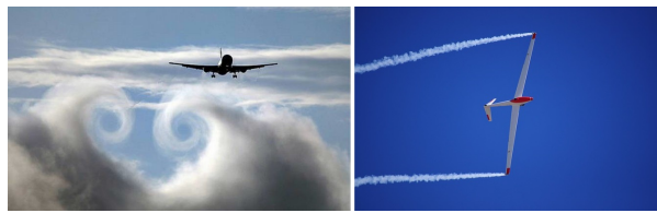
Figure 7. Illustration of marginal eddies at wingtips. On the left, the winding of these eddies generated by a large aircraft is made visible by the cloud below it. On the right, at the ends of the wings of a glider, these eddies are made visible by a condensation phenomenon located near their axis [Source: (left image) DR. (right image) Pixabay]
