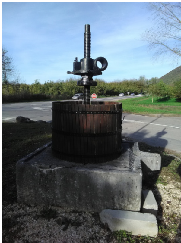
Figure 6. Grape press: in this case, the fluid is expelled radially: this is called radial consolidation. [Source: © Etienne Flavigny]
