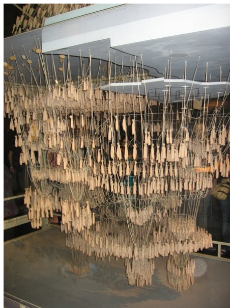
Figure 2. Inverted model of Gaudi's Sagrada Familia Cathedral. The equilibrium shape is such that at each wire intersection the vector sum of the forces is equal to zero. Each beam element is represented by a wire, and its mass simulated by a weight. The tension force on a yarn is necessarily aligned with the yarn. In the actual inverted configuration, the corresponding force will then be a compression force aligned along the beam, which guarantees its mechanical strength. [Source: http://olive-art.weebly.com/uploads/2/6/0/5/26053332/6555663_orig.jpg ].
