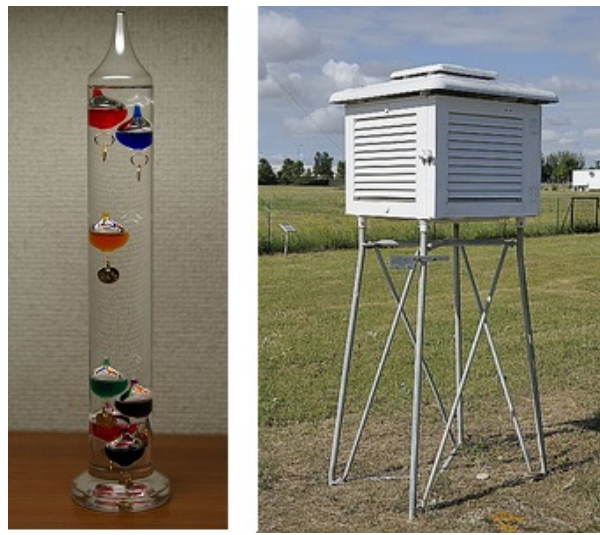
Figure 3. On the left, Galileo's thermometer [Source : By Hustvedt (Own work)]CC BY-SA 3.0 ( http://creativecommons.org/licenses/by-sa/3.0 ) via Wikimedia Commons]. On the right, a weather shelter to measure the air temperature
