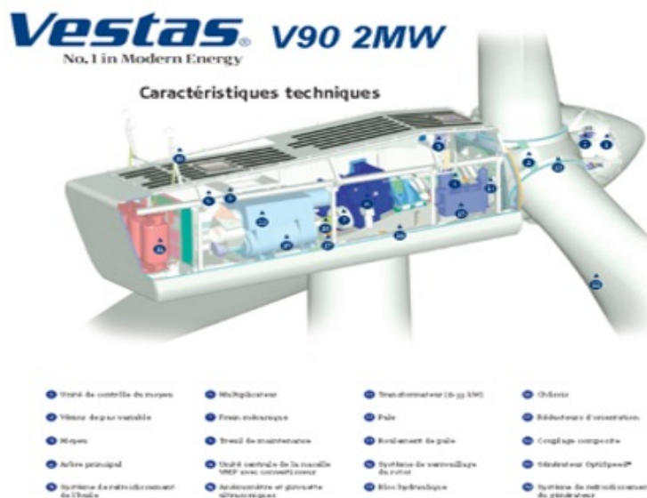
Figure 5. Exploded view of the VESTAS® nacelle - V90 - 2 MW [Source: © VESTAS]
