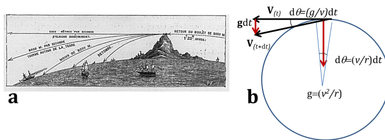
Figure 4. a) Movement of a launched body with increasing horizontal velocity, up to circular orbit satellite (8000 m/s) and Earth release (11 000 m/s) [Source: illustration of Newton's theory published in "Popular Astronomy"]. (b) Law of dynamics applied to the circular motion of a satellite: during a short time interval dt , the satellite rotates by an angle d\theta = (v/r)dt , and the velocity vector rotates by the same angle d\theta = (g/v)dt , from which g = (v^2/r) is derived.
