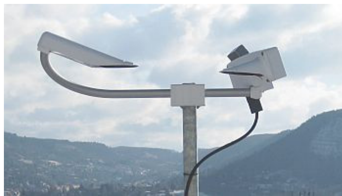
Figure 13. Present weather sensor. [Source : © Fabrice Zanghi]
