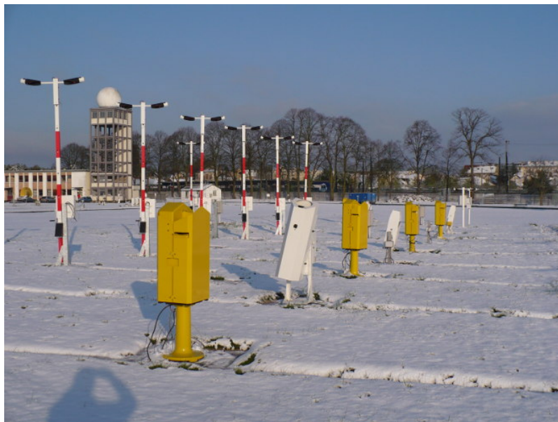
Figure 12. Cloud rangefinders. [Source : © Michel Leroy]
