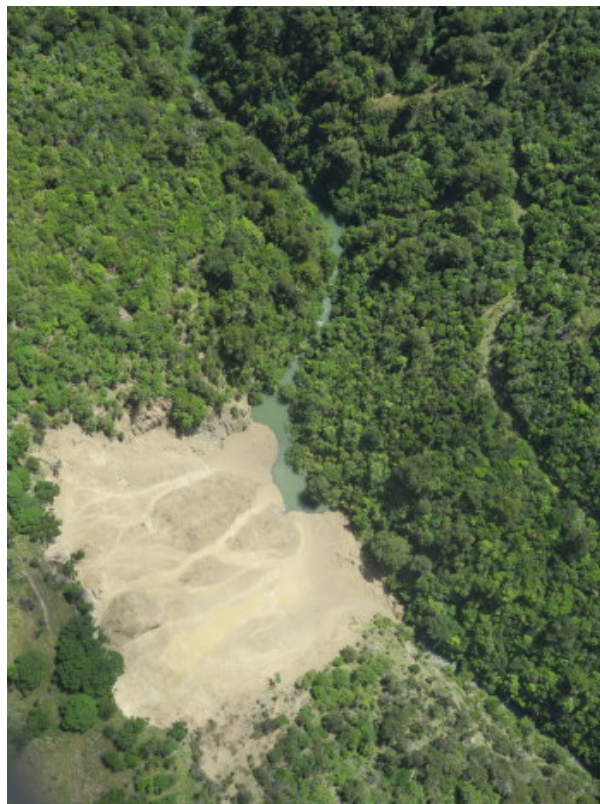
Figure 4. Natural dam and dam lake formed by obstructing the bed of the Ote Makura River from debris from a ground movement triggered by the 14/11/2016 earthquake in New Zealand. [© GNS Science (CC BY 3.0 NZ)]
