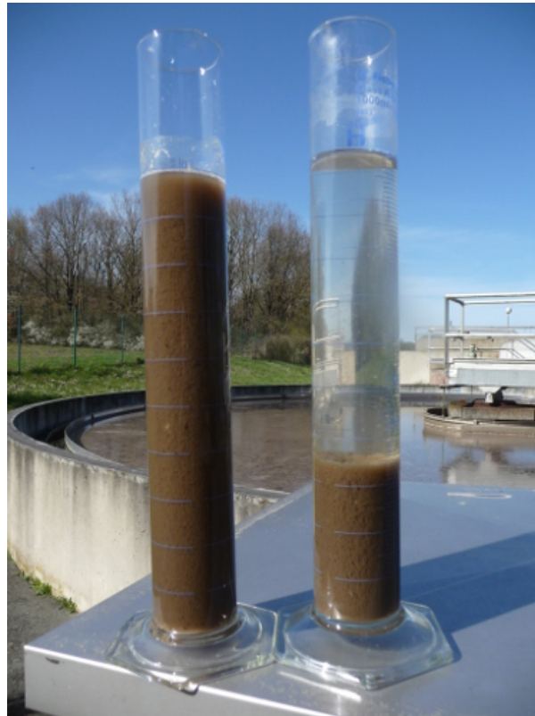
Figure 8. Biomass sample just taken from an activated sludge reactor (right sample) and after 30 minutes of settling (left sample). The supernatant represents treated water. [© Joseph De Laat]
