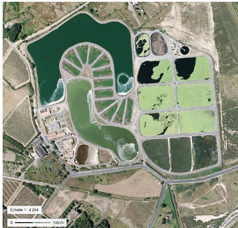
Figure 9. View of a natural lagoon treatment plant (Mèze site near the Thau pond) [Source: IGN - Geoportal]
