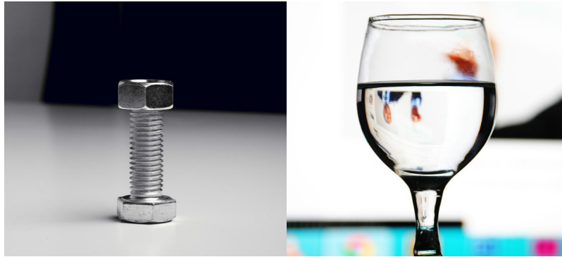
Figure 1. A metal block has its own shape: it is a solid; water takes the shape of the container that contains it: it is a fluid.
