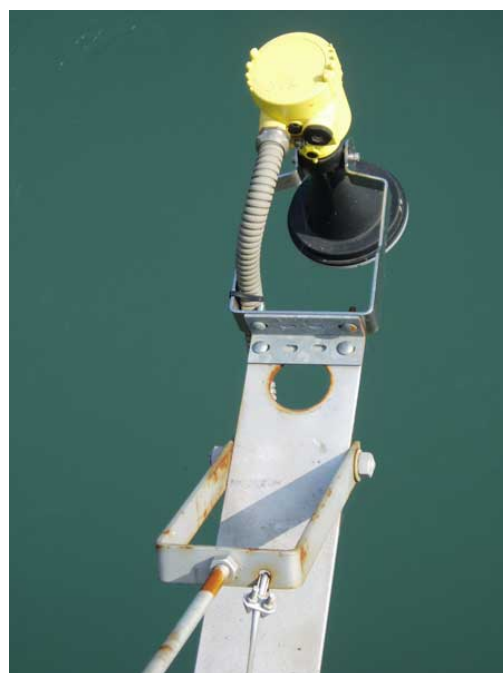
Figure 5. Level measurement by emerged radar. [© EDF DTG]
