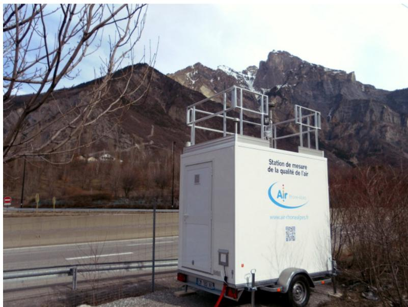
Figure 3. Station mobile de mesure des émissions. [Source : Air Rhône-Alpes [CC BY-SA 4.0 (<https://creativecommons.org/licenses/by-sa/4.0/>)]]
